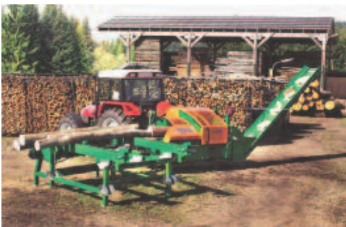
A combined cutting and splitting machine with conveyor belt.
