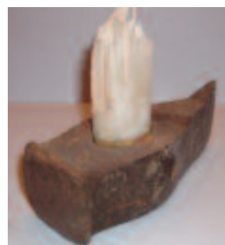
Figure 2: Steel splitting wedge. The head has been rounded after use to prevent splinters from flying off.
