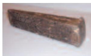
Figure 2: Steel splitting wedge. The head has been rounded after use to prevent splinters from flying off.
